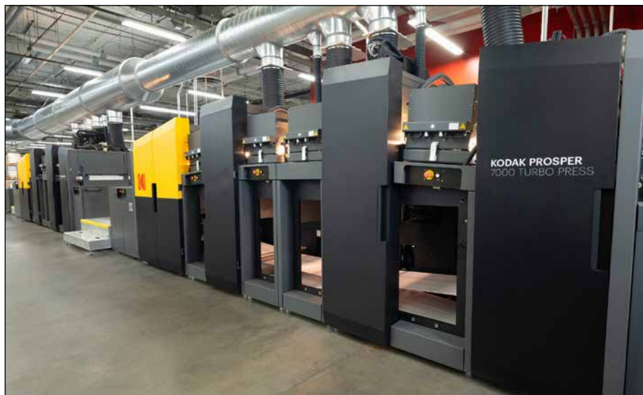
The Prosper 7000 Turbo Press is the world's fastest inkjet press, capable of printing at speeds of up to 410 mpm (1,345 fpm).
