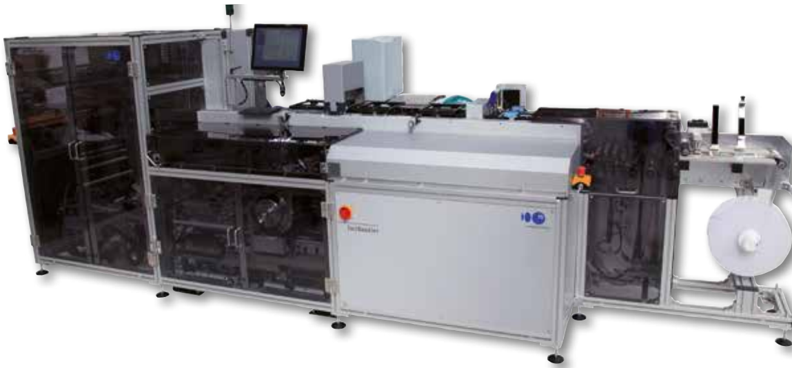
The fastBooklet machine from Imaging Solutions produces a complete lay-flat booklet direct from the roll in less than 30 seconds.
